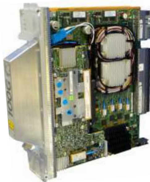
Figure 2 112 Gb/s, 50 GHz ITU grid compliant Co-FDM transceiver
