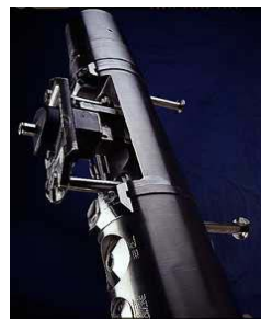
Figure 1. The formation tester tool in single-prove module
