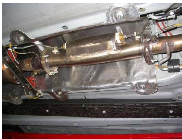
Fig. 2 The UV Gas Sensor Mounted Underneath the Car
